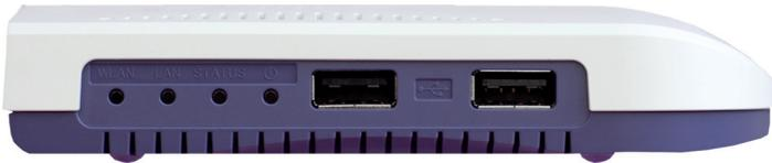
Two USB 2.0 Hi-Speed ports and control LEDs;
