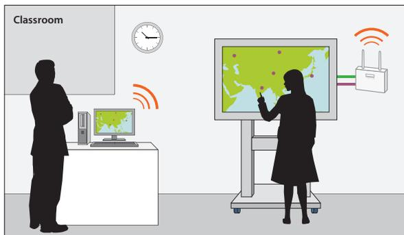
A wireless connection instead of cables next to the teacher's podium allows the whiteboard to be moved around the room without restriction, making it easier both to put away and to set it up.
