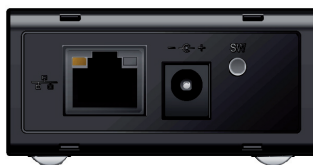
Fast Ethernet connection, reset button, power connection
